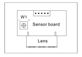
Remove the cover, and adjust the W1, turn clockwise to increase the distance, and counter clockwise to reduce the distance.
