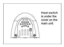
You can adjust warm or cool air via an internal switch. When it is turned on, it will produce warm air. When it is turned off, it will produce cool air.
