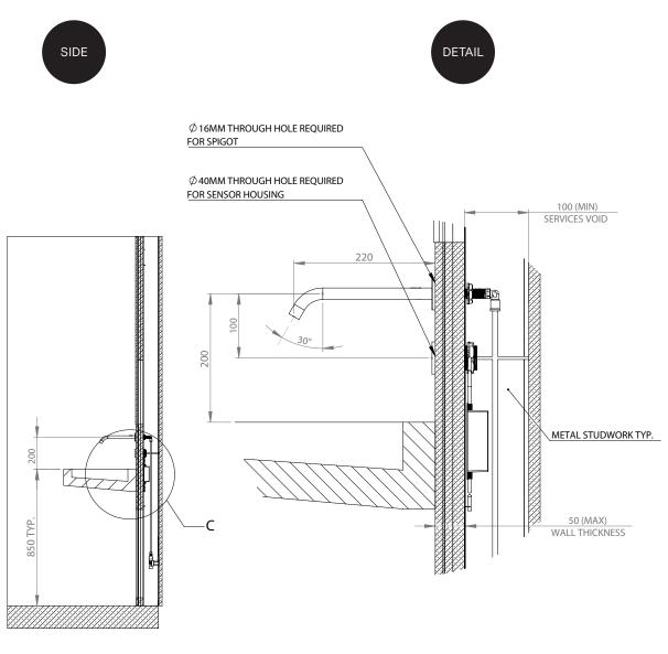
SECTION B-B DETAIL C SCALE 1:5
