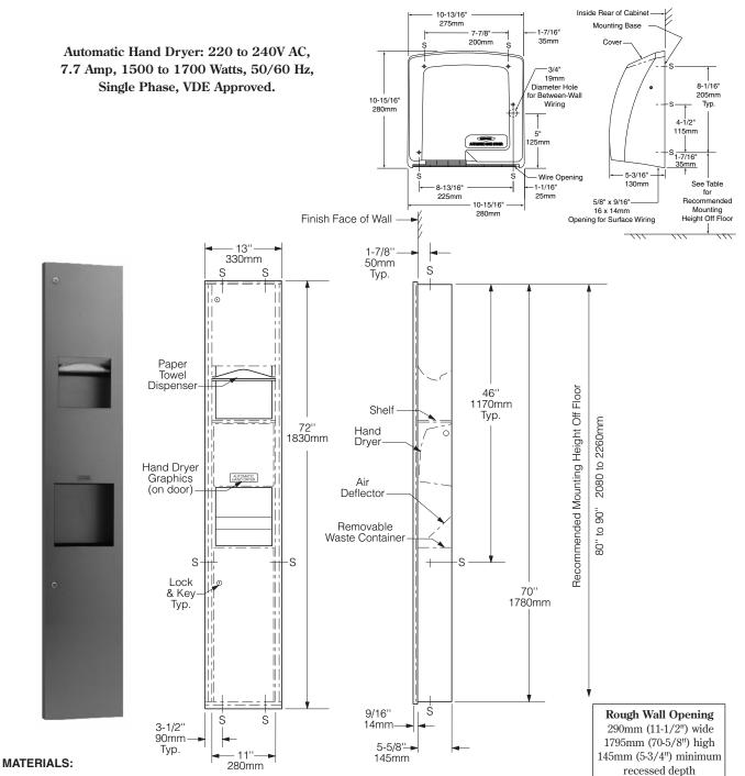
Cabinet — 18-8 S, type-304, heavy-gauge stainless steel. All-welded construction.
